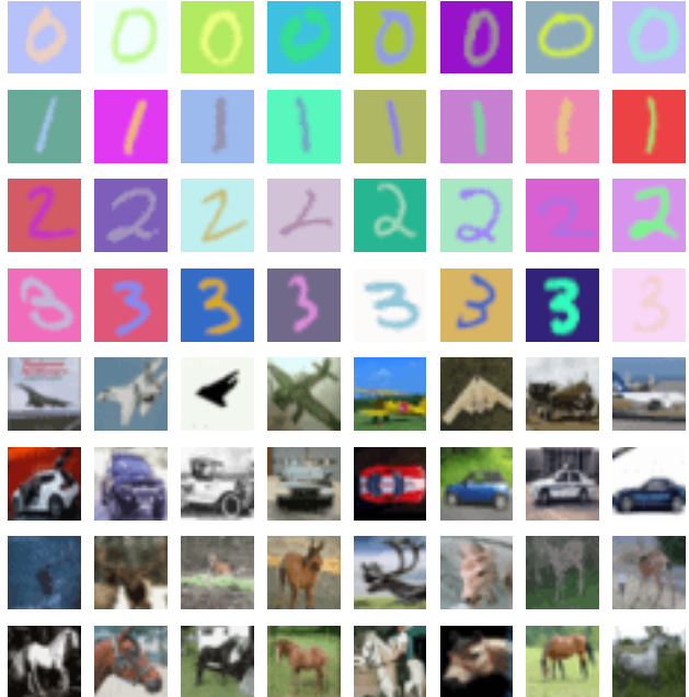
Figure 4. Sample images from the hybrid MNIST/CIFAR-10 dataset. We recolor images from MNIST via the following procedure: we select two random colors at least 0.3 units away from each other in RGB space; we then map black pixels to the first color, map white pixels to the second color, and linearly interpolate in between.
