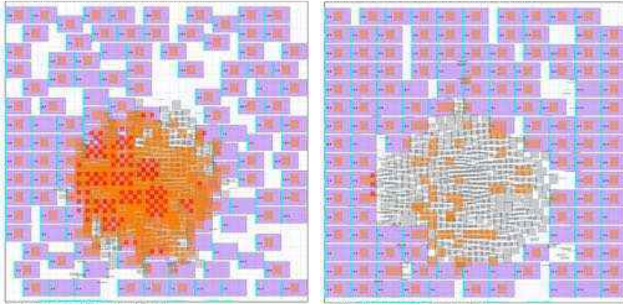
Figure 6. Visualization of placements. On the left, zero-shot placements from the pre-trained policy and on the right, placements from the finetuned policy are shown. The zero-shot policy placements are generated at inference time on a previously unseen chip. The pre-trained policy network (with no fine-tuning) places the standard cells in the center of the canvas surrounded by macros, which is already quite close to the optimal arrangement and in line with the intuitions of physical design experts.
